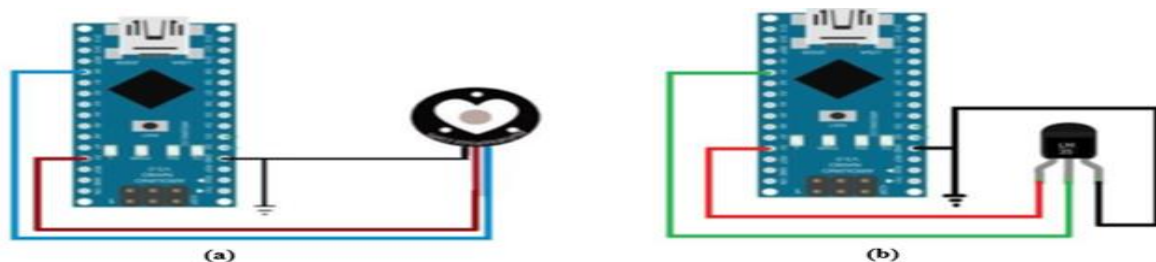
Fig. 3: Circuit Configuration of (a) heartbeat sensor and (b) body temperature sensor (LM35) with Arduino Uno
